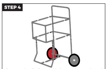
Flip top portion of ball cart upside down on the ground. Attach bottom portion of ball cart to pre-assembled top portion. NOTE: If frame is tight you may use a Rubber Mallet to gently
