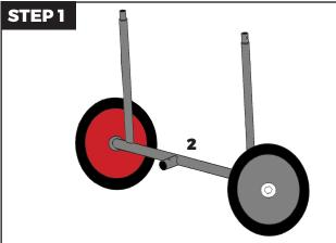
Slide (2) Never Flat Wheels to Bottom frame wheel assembly (Part #2). Place protective wheel plate over wheel hub and attach pre-installed lock washer and bolt.
