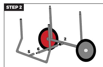
Join Front Leg assembly (Part #5) to Part #2 using Bottom center piece (Part #6) via push button assembly provided.
