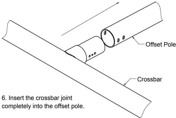
6. Insert the crossbar joint completely into the offset pole.
