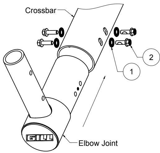
8. Insert the elbow joint into the crossbar and secure it with serrated washers and flange bolts.
