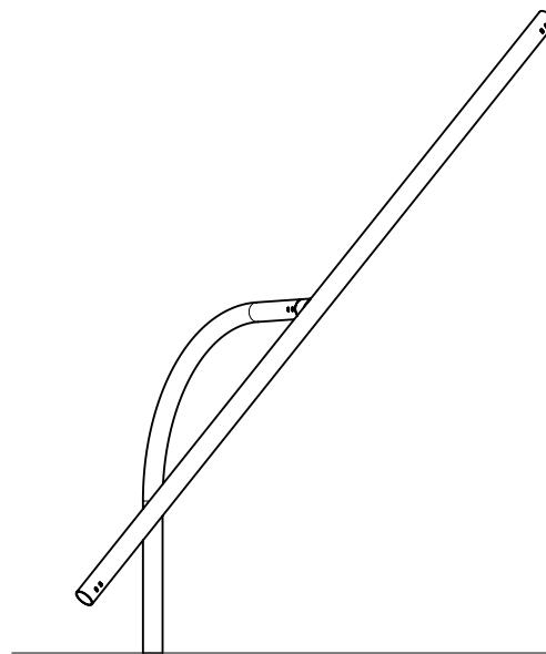
7. With caution tilt the crossbar to bring one end down to a few feet above ground level.
