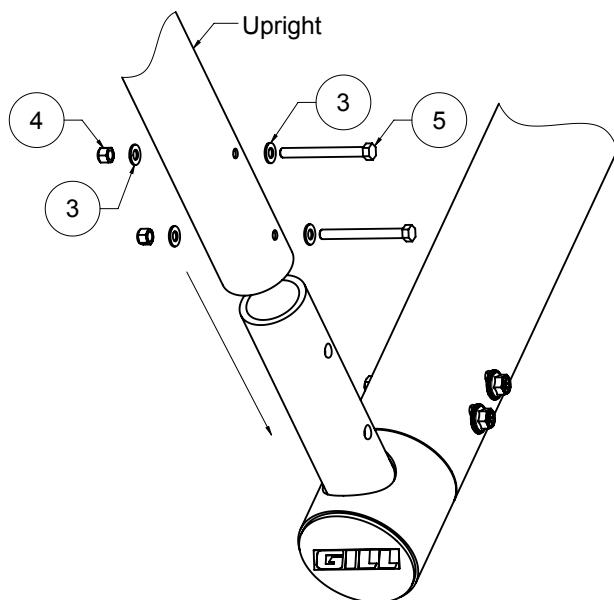
9. Slide the upright onto the elbow joint and secure it with bolts, washers, and nylock nuts.
