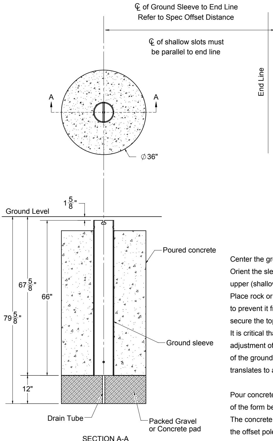
Local soil conditions will determine the actual size of concrete foundations. The following instructions are recommendations only, and should be considered minimums.
