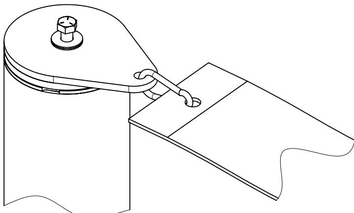
Install the flags onto the tops of the uprights BEFORE installing the uprights onto the crossbar.
