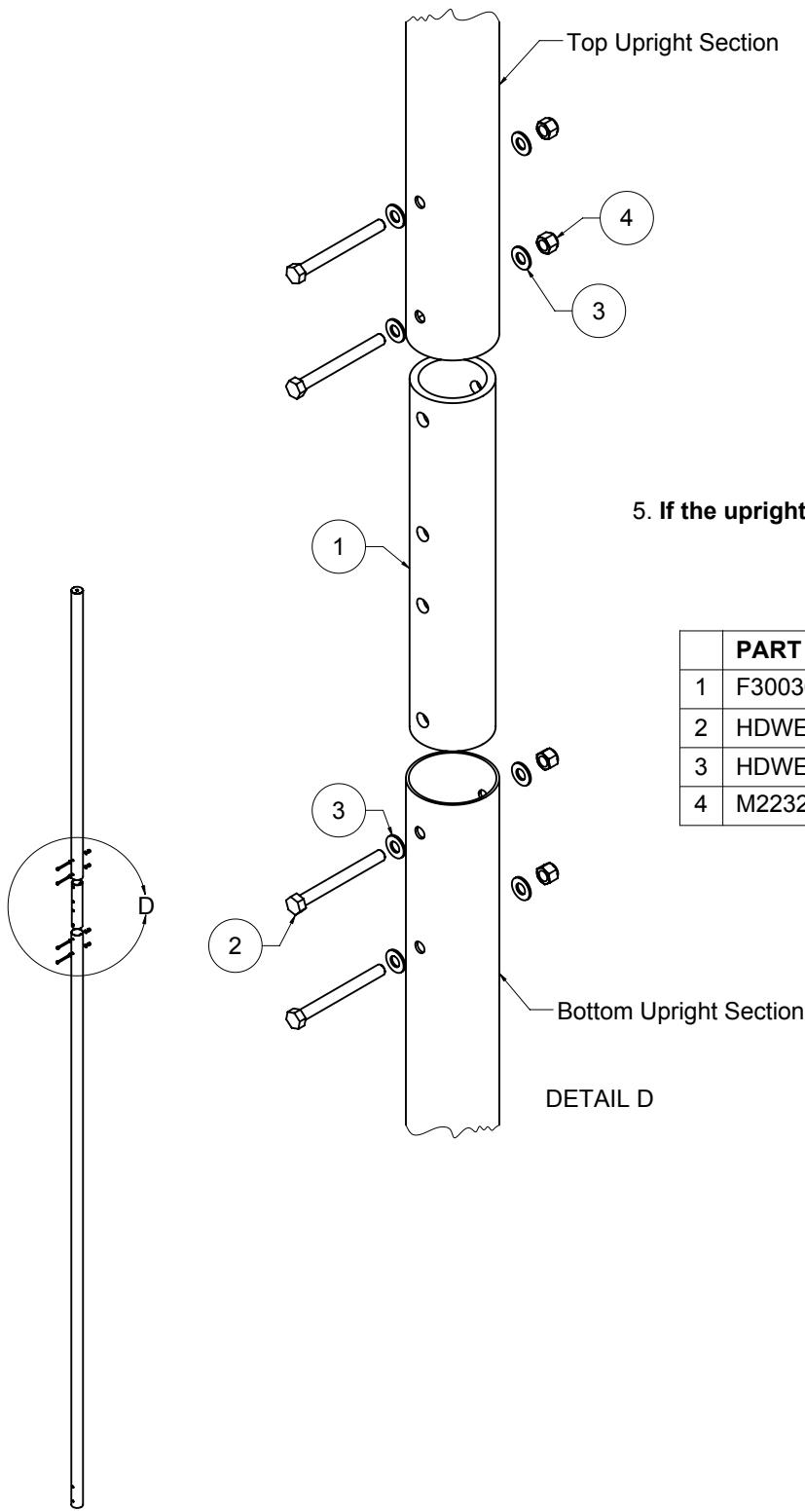
5. If the uprights are spliced, assemble the uprights with the splice tubes.
